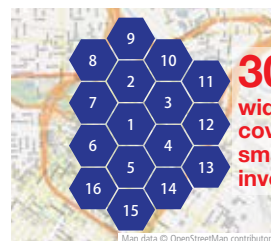
6.25 kHz At a total of 2150 sq. miles coverage: 6.6-mile radius per site / only 16 site total
